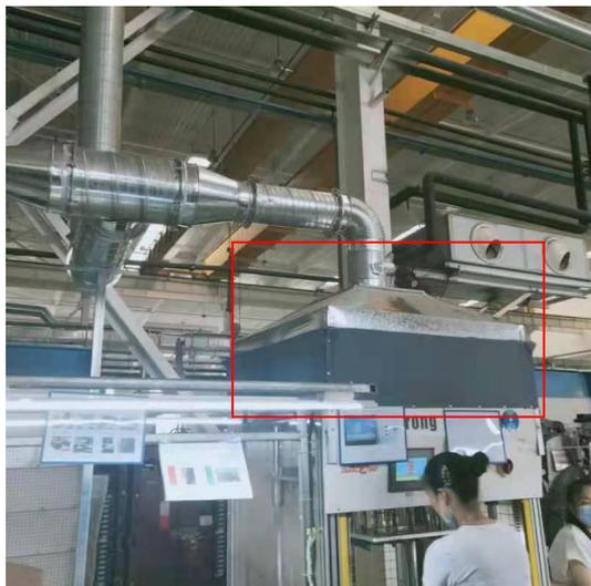
热铆焊接工序废气集气罩
