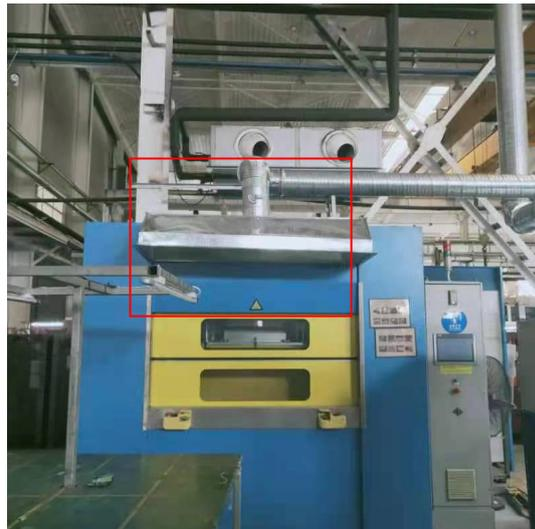
震动摩擦焊接工序废气集气罩
